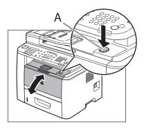
If you are using the multi-purpose tray, close it before opening the front cover. To open the front cover, push the open button (A).
